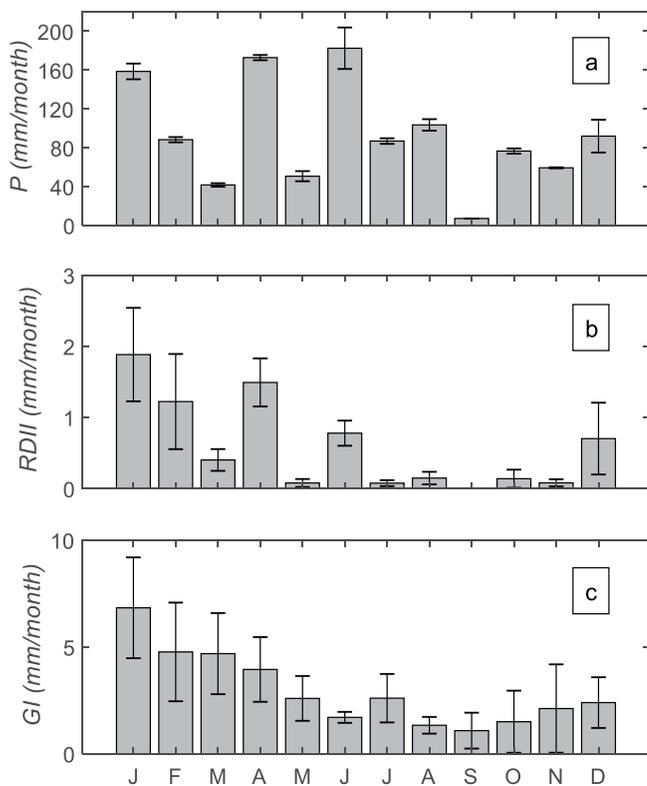
**Figure 4.** Variations in (a) total-monthly precipitation, (b) rainfall-derived infiltration and inflow, and (c) groundwater infiltration averaged among all monitoring locations. Error bars indicate the standard deviation among measurement locations.
