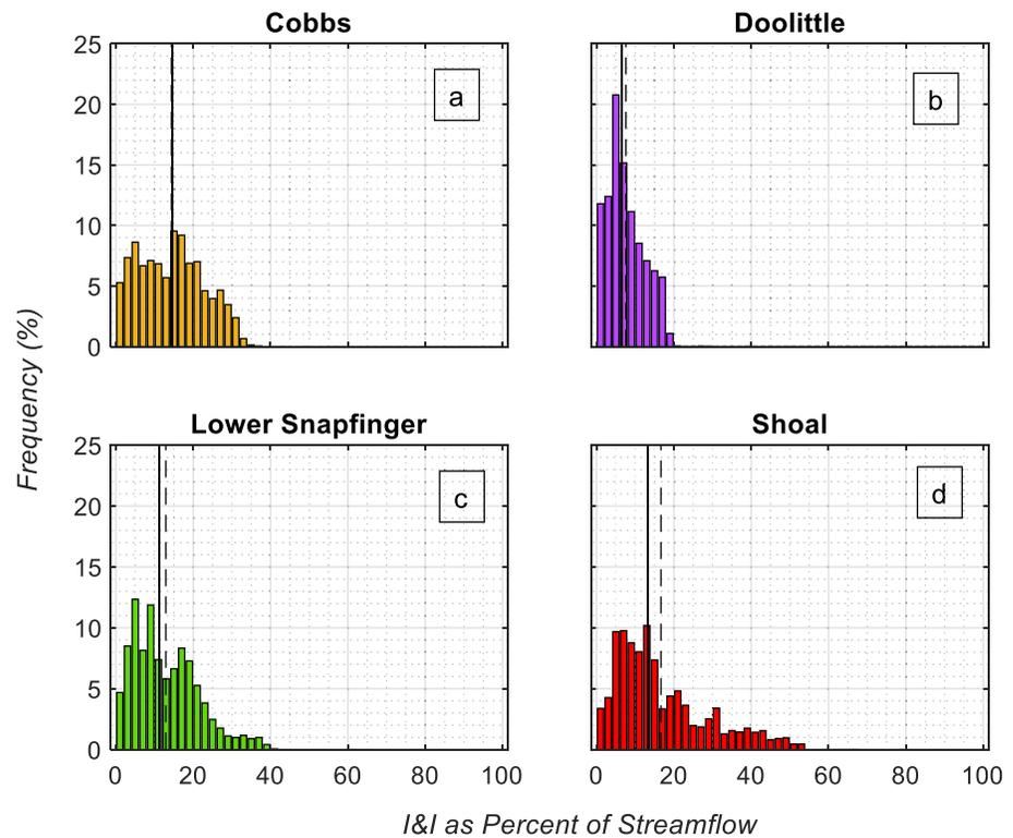
**Figure 6.** Frequency distributions of I&I expressed as a percentage of streamflow measured in the nearby channel. Both variables are quantified at 15-min intervals. The vertical axis represents the percent of all measurements taken in 2019 at that time interval. Bar colors correspond to the colors used to represent pipe networks in each watershed in Figure 1. The solid and dashed black lines indicate the median and mean of the distributions, respectively.
