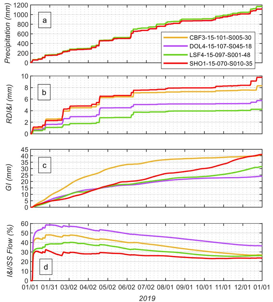
**Figure 3.** Time series of (a) cumulative precipitation, (b) cumulative rainfall-derived I&I, (c) cumulative groundwater infiltration, and (d) total I&I (RDI&I + GI) divided by total sanitary-sewage flow. All cumulative flows are divided by the respective watershed area and reported as area-normalized depth (mm). Legend entries correspond to the monitor identification codes shown in Table 1. Line colors correspond with colors used to represent pipe networks for each watershed within Figure 1.
