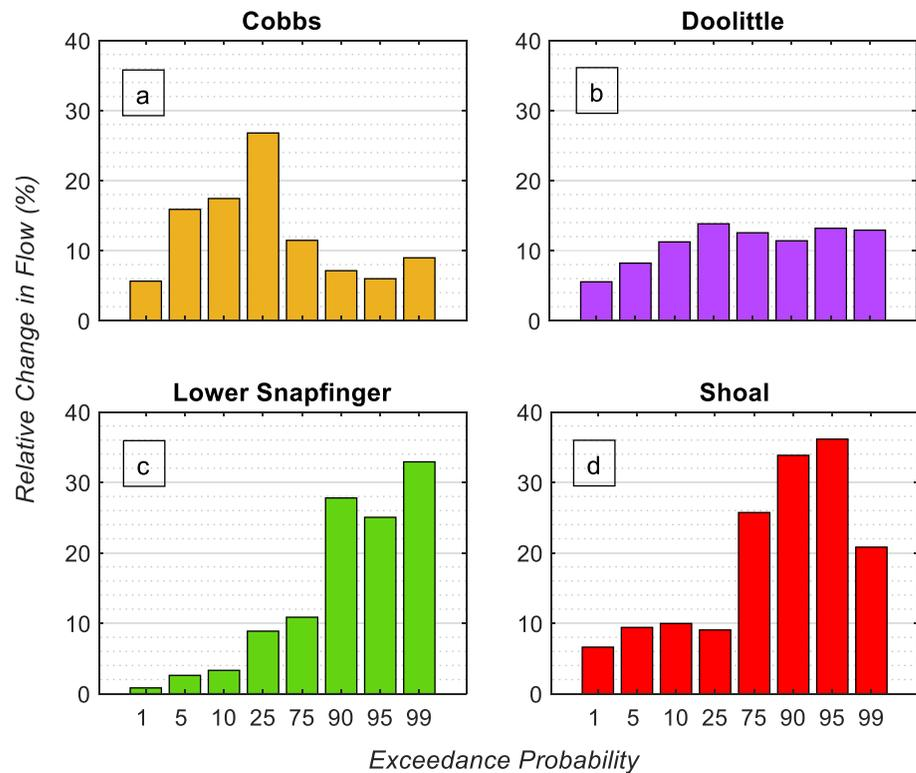
**Figure 8.** The vertical axis shows the potential, relative increase in streamflow magnitude that would be possible if no I&I occurred, and all associated water was instead discharged into local stream channels. The horizontal axis values correspond to selected probabilities from the cumulative probability distributions of flow exceedance (e.g., as shown in Figure 7).
