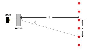
In the figure above the diffraction pattern due to the mesh is seen on the right. The angle  $\theta$  is shown for the m = 2 peak (second peak from the central peak).  $\theta$  can be determined from measurements of x and L.
