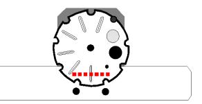
the laser until you see a clear, horizontal diffraction pattern on the white screen of the aperture bracket.
