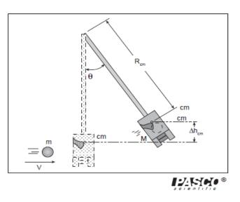
This exercise illustrates the concepts of **conservation of energy** and **conservation of momentum**, and uses a type of device (the **ballistic pendulum**) originally invented for determining the speed of a bullet.
