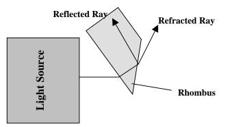
3. Rotate the ray table until the emerging ray just barely disappears. Just as it disappears, the ray separates into colors. The table is rotated far enough if the red color has just disappeared.
