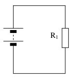
2. Break the circuit and connect the ammeter in series at the place where the current will be measured.
