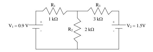
Using the cautions and methods of measurement described in 2 and 3, measure  $V_1$ ,  $V_2$ , and  $V_3$  as well as  $I_1$ ,  $I_2$ , and  $I_3$ .
